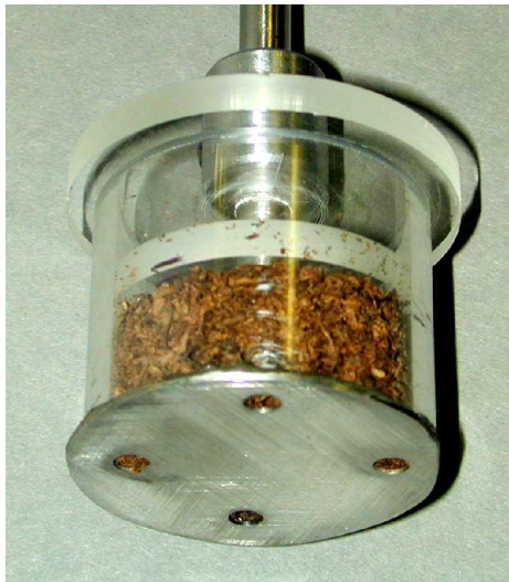
Figure 6. Close up of the new sample holder, with the plunger and lid assembly, used to compress the samples to a precise depth, still in place.
