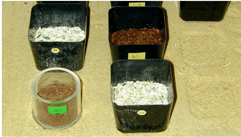
Figure 5. Rooting media samples on a sandbed for a drainage experiment. The sample at the front left is in one of the new sample holders made from Perspex tube, the others are the original sample holders made from the base of 7 cm square plastic pots.
